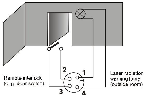
**Figure 3: Remote Control Interlock**
